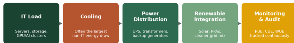
Figure 4.1 — Where a Data Centre's Energy Actually Goes
